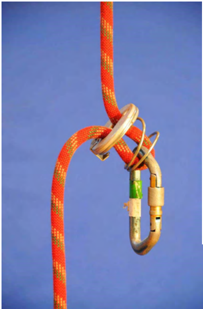
The first of the belay devices. The Salewa Stitch Plate. It revolutionised climbing. It is an aperture device.
