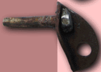
FILED DOWN HAMMER IN MACHINE BOLT 'CARROT' 9mm x 50mm WITH HOMEMADE NON-SS HANGER
