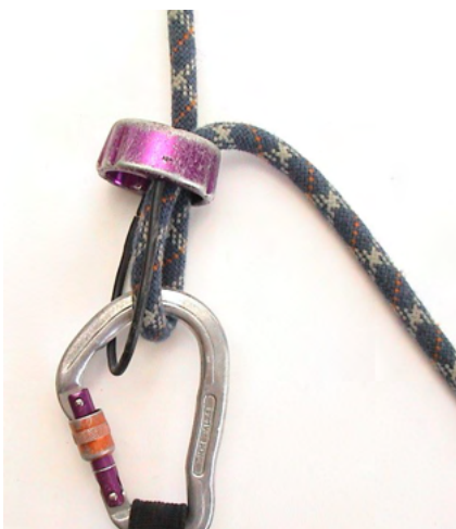
ATC/ Tubular belay device. Not easily locked off. Heats up quickly. Can be very jerky.
